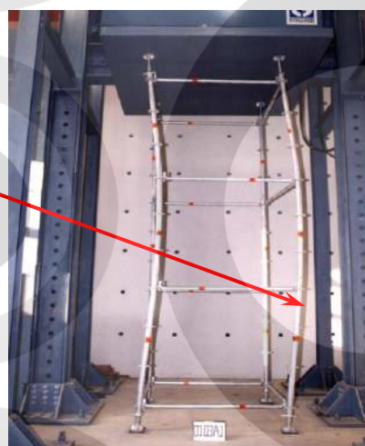
(2) The experiment of no Diagonal for three layers
