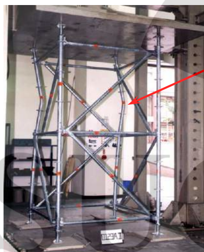
(3) The experiment of erected Diagonals for two layers
